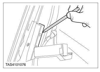
4. Using a suitable marker pen, mark the position of the hinges.
