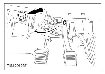
3. Remove the servo push rod clip.
