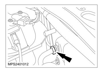
6. Disconnect the upper transmission fluid hose (if fitted).
