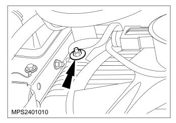
12. Remove the left-hand fan shroud retaining nut.
