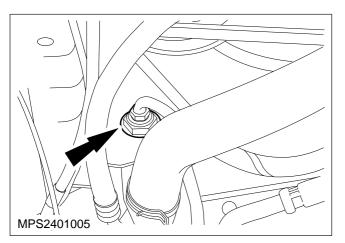
3. Disconnect the lower transmission fluid hose (if fitted).
