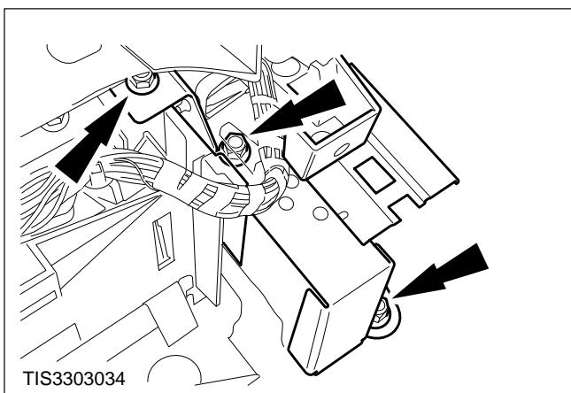
**7. Detach the PATS module.**
