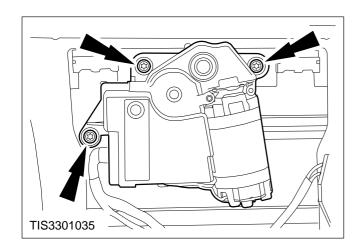
4. Remove the motor (three bolts).
