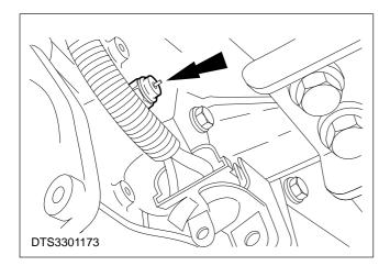
4. Disconnect and remove the oil pressure switch.
