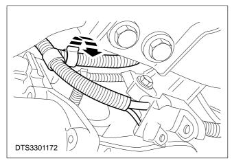
3. Detach the wiring harness from retaining clip.
