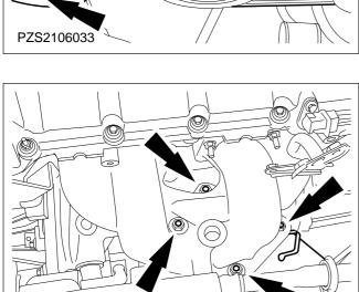
24. Detach the catalytic converter from the exhaust manifold.
