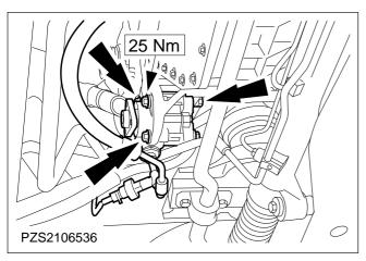
81. Attach the bracket to the catalytic converter and the automatic transmission.
