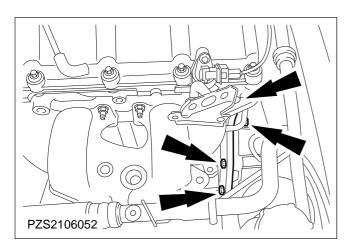
38. Detach the steering intermediate shaft.
