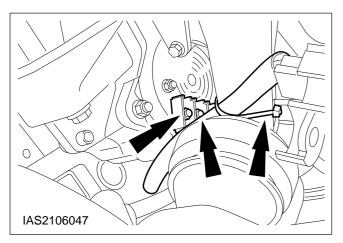
34. Detach the bracket for the oil pipes.
