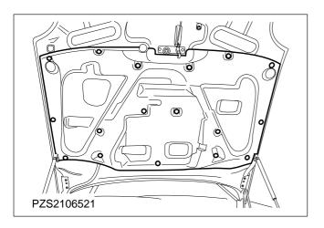
104. Fit the hood insulation panel (17 expanding pins).
