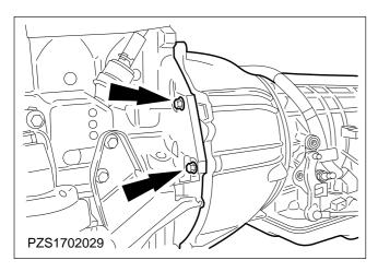
53. Remove the starter motor and bracket.
