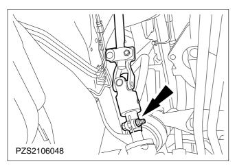
42. Detach the oil dipstick tube and the earth lead.
