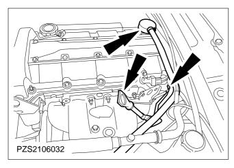
19. Disconnect the heated oxygen sensor (HO2S) plug.
