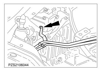
40. Disconnect the starter motor lead.
