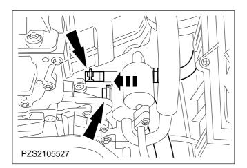
111. Attach the coolant hoses to the coolant pump.
