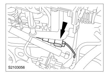
8. Connect the fuel shut-off valve electrical connector.
