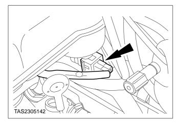
27. Disconnect the engine coolant low level warning switch multiplug.
