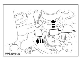
14. Disconnect the accelerator cable from the fuel lever.
