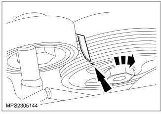
32. Turn the engine clockwise until number one cylinder is at TDC.
