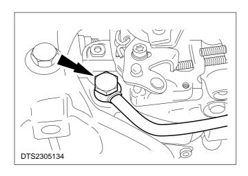
19. Disconnect the fuel supply pipe from the fuel injection pump.
