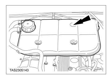
28. Remove the three retaining screws and position the expansion tank to one side.
