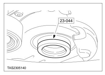
11. Install the special tool adaptor to the timing cover.
