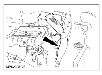
4. Remove the air cleaner outlet tube.
