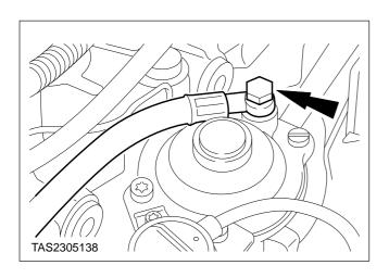
23. Disconnect the vacuum pipe from the exhaust gas recirculation vacuum regulator.
