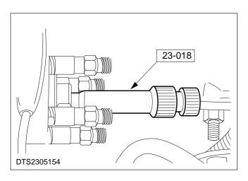
50. Install the dial gauge holding fixture to the rear of the fuel injection pump.
