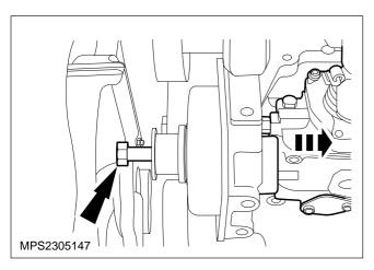
39. Fit the bolt to the special tool and extract the fuel injection pump from the drive gear.
