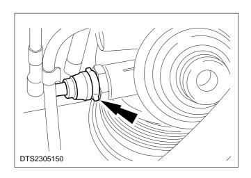
Fuel Injection Pump – Timing – Check 23 410 0
