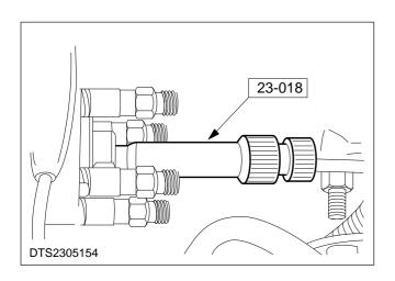
34. Install the dial gauge holding fixture to the rear of the fuel injection pump.
