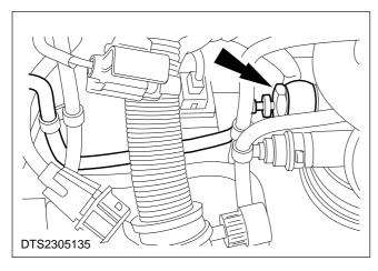
20. Remove the fuel supply pipe.
