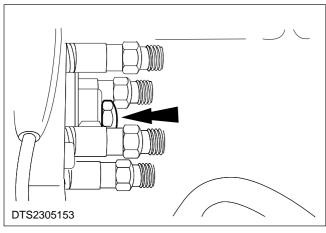
49. Remove the blanking plug from the rear of the fuel injection pump.
