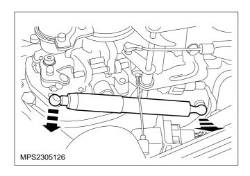
15. Remove the fuel lever damper.
