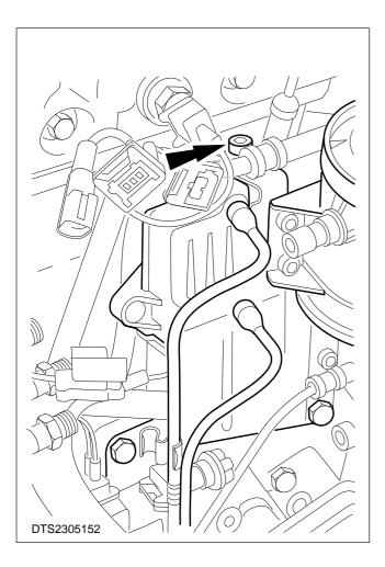
48. Remove the four retaining bolts and position the diesel fuel heater mounting bracket to one side.
