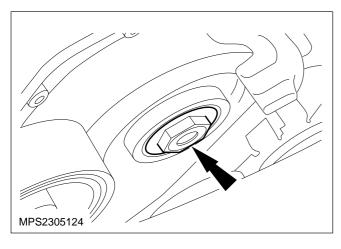
45. Install the blanking plug to the timing cover.
