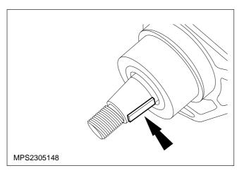
**NOTE:** When installing the fuel injection pump make sure that the key in the shaft locates in the correct keyway in the fuel injection pump drive gear.
