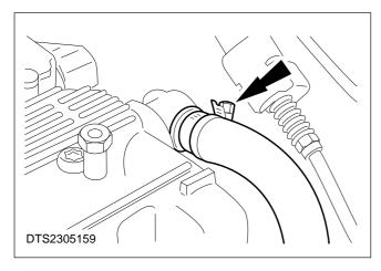
30. Disconnect the vent pipe from the cam cover.
