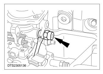
21. Disconnect the fuel return pipe from the fuel injection pump.
