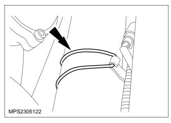
3. Remove the air cleaner outlet tube retaining band.
