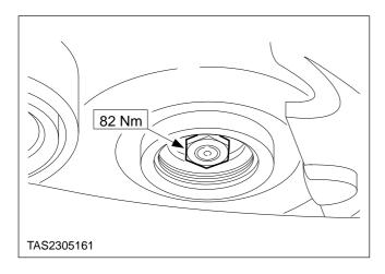
44. Install the fuel injection pump drive gear retaining nut and locking washer.
