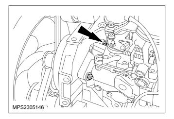
38. Remove the fuel injection pump retaining nuts.
