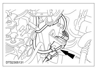
16. Detach the three fuel injection pump multiplugs from the bracket and disconnect them.
