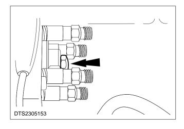
33. Remove the blanking plug from the rear of the fuel injection pump.
