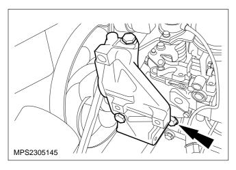
26. Remove the alternator drive belt idler pulley/air conditioning compressor/alternator assembly mounting bracket.
