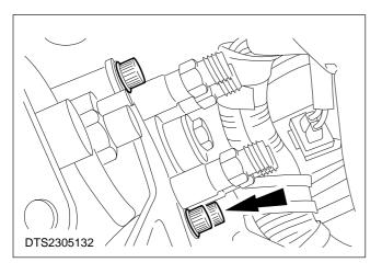
17. Remove the three fuel injection pump bracket retaining bolts.
