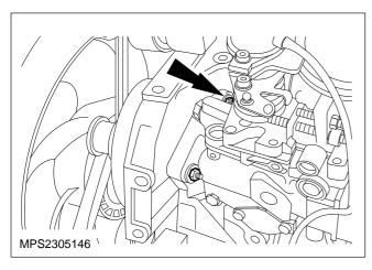
Fuel Injection Pump – Timing – Adjust 23 411 0
