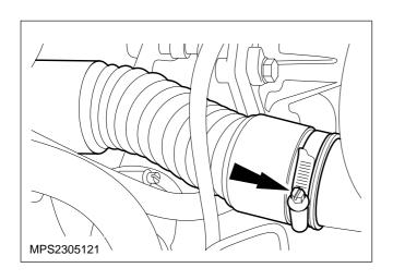
2. Disconnect the air cleaner outlet tube from the turbocharger compressor intake pipe (one clip).
