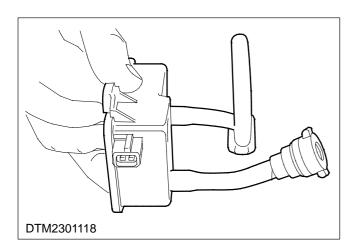
4. Remove the diesel fuel heater.
