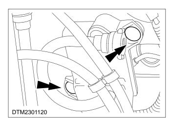
3. Carefully prise out the fuel heater retaining pins.
