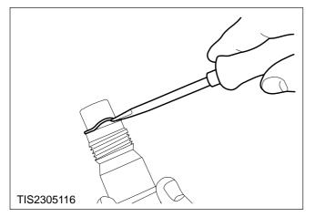
10. Disconnect the fuel injector return pipes.
