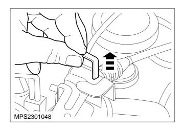
4. Remove the outer cable retaining clip.
