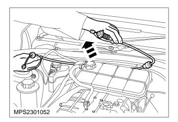
8. Remove the accelerator cable.
