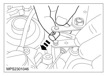
2. Remove the inner cable retaining clip.
