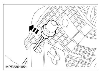
7. Unclip the inner cable from the accelerator pedal.
