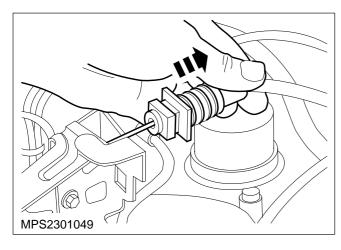
5. Disconnect the outer cable from the bracket.
