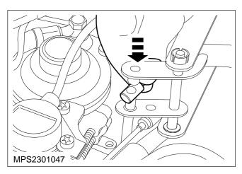
3. Disconnect the inner cable from the injection pump mechanism.
