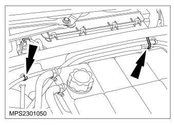
6. Cut the cable ties which secure the outer cable to the bulkhead.
