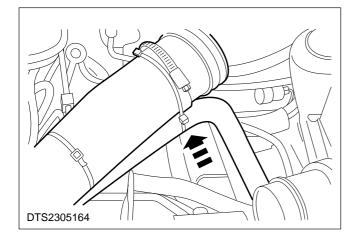
3. Position the air cleaner outlet tube to one side.
