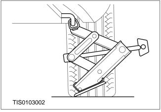
The owner jack should be located on the provided pin in the wheel housing at the ends of the rocker panels.
