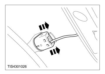
5. Slide the mirror towards the roof to disengage it from its bracket and remove.
