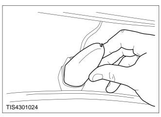
4. Unclip and remove the mirror bezel.
