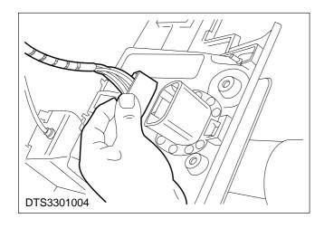
**NOTE:** There is no need to disconnect the hood release cable when detaching the diagnostic connector.
