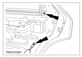
5. Remove the lower rear glass guide channel (two screws).
