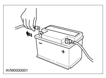
9. Disconnect the battery negative lead.
