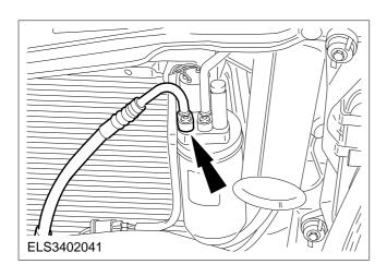
7. Disconnect the line from the condenser at the accumulator/dehydrator.
