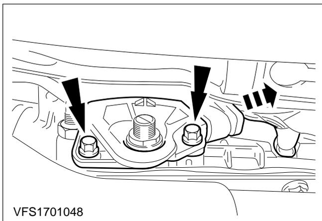
**8. Disconnect the plug of the TR switch and remove the TR switch.**
