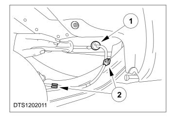
5. Detach the handbrake cable from the lower arm.
