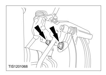
6. Remove the brake caliper assembly.
