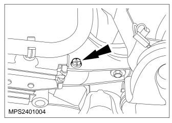
3. Drain the cooling system into a suitable container.
