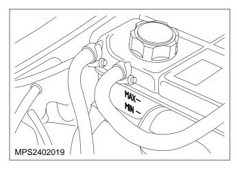
10. Check the coolant level and top up to the maximum mark if necessary.
