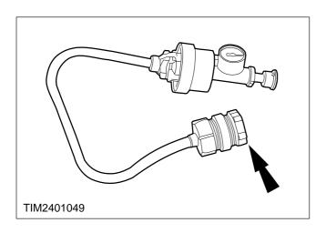
7. Fit the appropriate pressure test adaptor to the cap and assemble on the tester.
