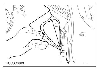
CAUTION: When detaching the foam watershield avoid touching the adhesive surface as rebonding will be impaired.
