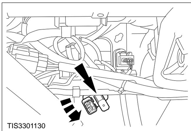
**4. Remove the de-activator switch.**
