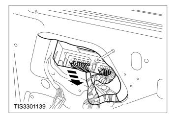
6. Slide the module sideways to release and manoeuvre the module out through the aperture.
