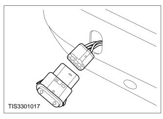
Switch – Front Seat – Height Adjuster – Remove (33 585 0)
