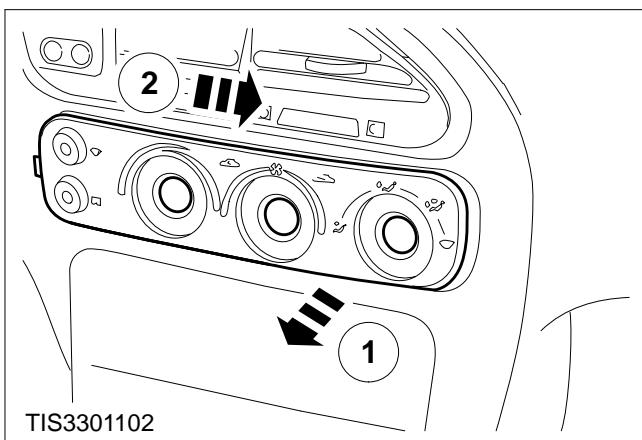
**4. Remove the heater control bezel from the instrument panel facia.**
