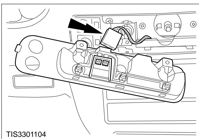
**5. Disconnect the multiplug and remove the heater control bezel.**
