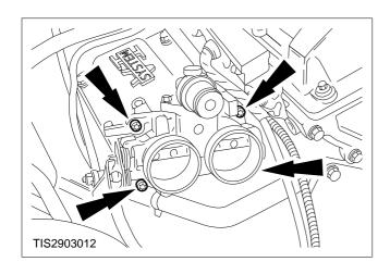
8. Unscrew the four throttle body Torx retaining screws.
