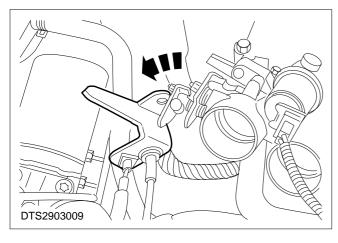
5. Lift the accelerator cable bracket to one side.
