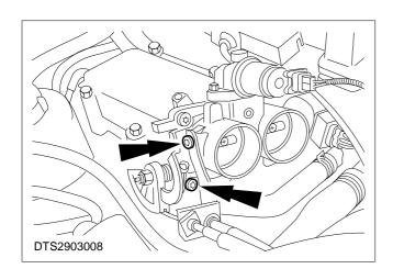
4. Unscrew the two accelerator cable bracket Torx retaining screws.
