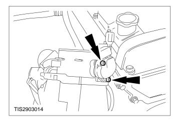
10. Unscrew the TP sensor Torx retaining screws.
