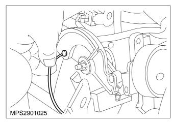
5. Disconnect the accelerator cable from the throttle body.
