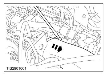
3. Slacken the clip and disconnect the intake hose.
