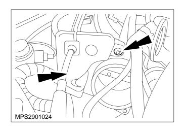
4. Unscrew the accelerator cable bracket retaining bolts.
