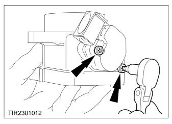
10. Unscrew the TP sensor retaining bolts.
