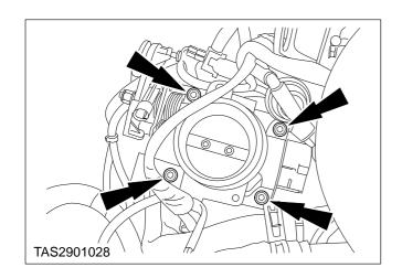
8. Unscrew the throttle body retaining bolts.
