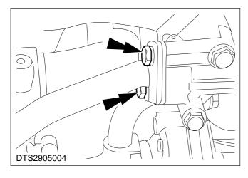
3. Unscrew the exhaust manifold to EGR valve pipe retaining bolts.
