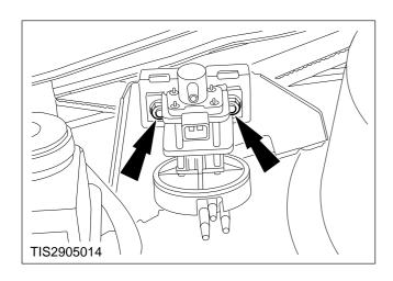
4. Unscrew the electronic vacuum regulator retaining bolts.
