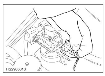
CAUTION: Do not pull on the wiring; pull on the multiplug body.
