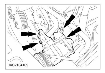
10. Remove the air conditioning compressor.
