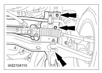
18. Unscrew the two lower engine mountings (one nut on each side).
