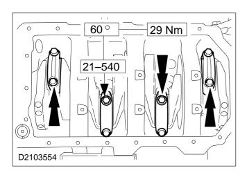
**NOTE:** The corresponding numbers on the connecting rods and the bearing caps point towards the camshaft side.
