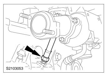
**NOTE:** Escaping fuel. Close off the openings in the injection pump and the injectors with suitable plugs.
