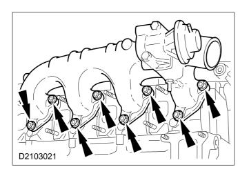
**NOTE:** Do up the retaining nuts lightly to align the cylinder heads.
