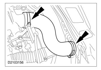
7. Remove the air hose between the inlet manifold and the intercooler.
