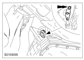
27. Detach the crankshaft locking tool from the crankcase intermediate flange.
