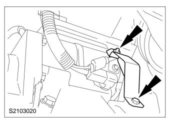
19. Detach the heat shield bracket from the starter motor.
