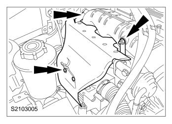
8. Remove the turbocharger heat shield.
