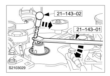
24. Remove the crankshaft front oil seal.
