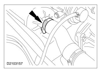
42. Attach the intake pipe to the turbocharger.
