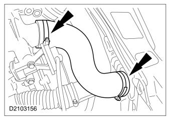
41. Air hose between the intake manifold and the intercooler.
