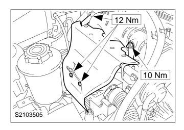
39. Attach the turbocharger heat shield.
