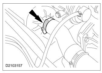
9. Detach the intake pipe from the turbocharger.
