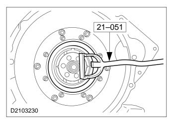
3. Remove the crankshaft position (CKP) sensor.
