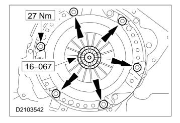
11. Centre the clutch disc on the pressure plate.
