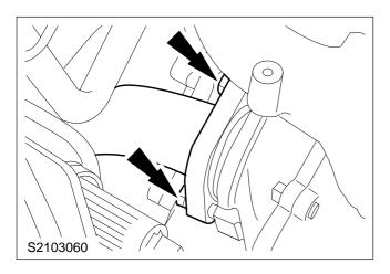
12. Detach the intake pipe from the turbocharger.
