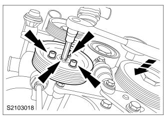
30. Detach the oil pipes from the oil cooler.
