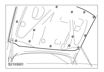
92. Fit the hood insulation panel (15 clips).
