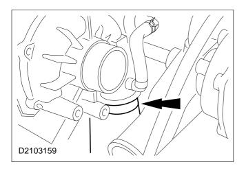
79. Push the vacuum line onto the brake servo vacuum pump.
