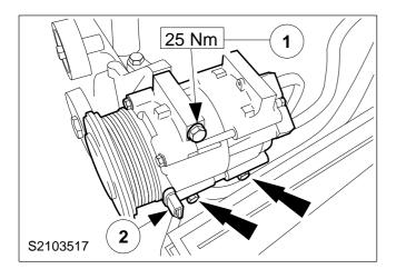
61. Install the power steering pump.
