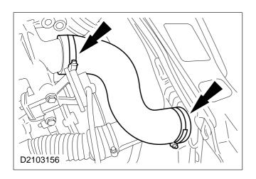
11. Remove the air hose between the inlet manifold and the intercooler.
