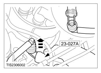
4. Disconnect the fuel return pipe from the fuel pressure regulator.
