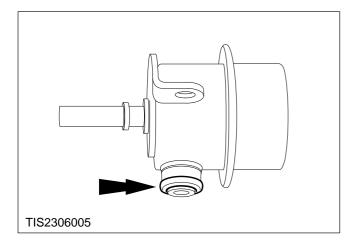
5. Disconnect the vacuum pipe from the fuel pressure regulator.
