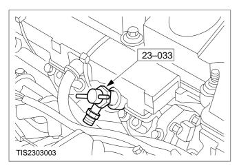
WARNING: Ensure that the tap on the tool is turned fully anti-clockwise before fitting and be prepared for some fuel spillage. Observe fuel handling precautions.
