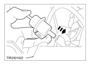
9. Disconnect the fuel hose and remove the fuel pressure regulator.
