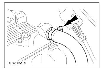
20. Disconnect the engine coolant low level warning switch multiplug.
