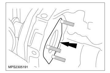
39. Disconnect the fuel return pipe from the fuel injection pump.
