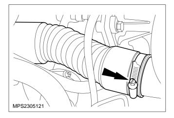
2. Remove the air cleaner outlet tube retaining band.
