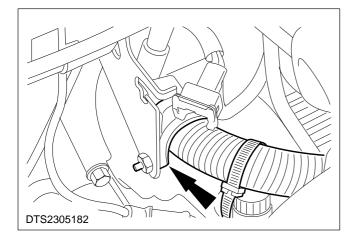
16. Disconnect the stop control solenoid electrical connector.
