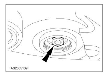
34. Remove the fuel injection pump drive gear retaining nut.
