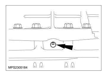
**NOTE:** After aligning the TDC mark, check the positioning of the valves as there are two holes in the flywheel.
