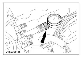
51. Remove the blanking plug from the rear of the fuel injection pump.
