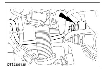
35. Install the special tool adaptor into the timing cover.
