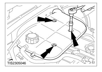
2. Remove the three expansion tank retaining screws.
