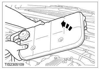
3. Position the expansion tank to one side.
