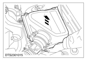
4. Unscrew the intake pipe retaining screw.
