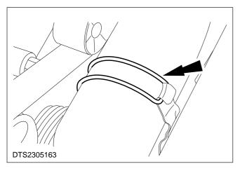
2. Remove the air cleaner outlet tube retaining band.
