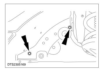
10. Remove the air cleaner retaining nuts.
