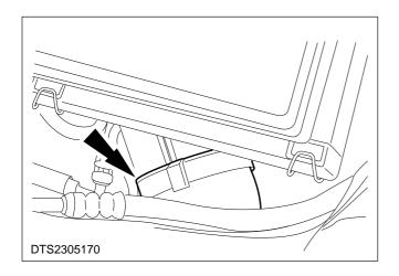
12. Disconnect the air cleaner inlet tube.
