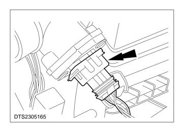
4. Disconnect the mass air flow sensor electrical connector.
