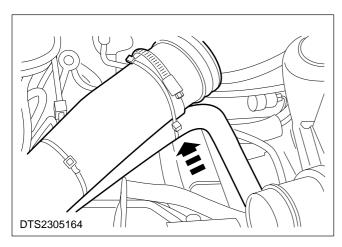
3. Position the air cleaner outlet tube to one side.
