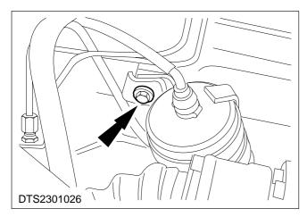
3. Unscrew the fuel filter bracket retaining bolt.
