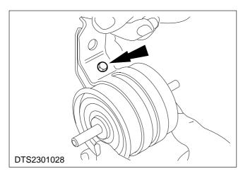
5. Unscrew the fuel filter clamp bolt.
