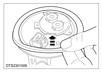
4. Remove the fuel pump/sender unit locking ring.
