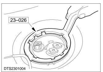
3. Release the fuel pump/sender unit locking ring.
