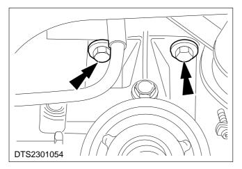
4. Unscrew the bolts and remove the filter head.
