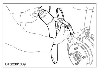
10. Remove the fuel tank filler pipe.
