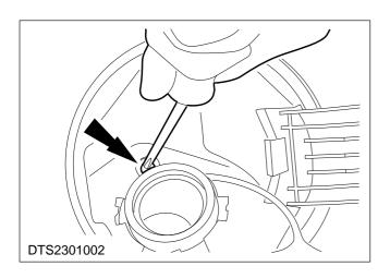
7. Unscrew the fuel tank filler pipe retaining screw.
