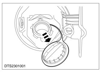
6. Remove the fuel tank filler cap.
