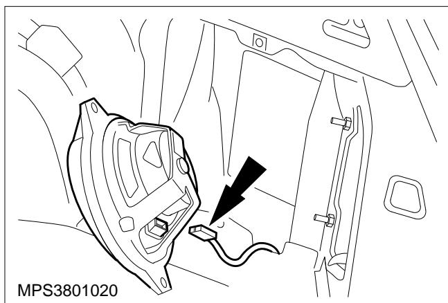
**! CAUTION:** When disconnecting multiplugs do not pull on the wiring; pull on the multiplug body.
