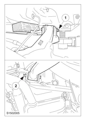
**NOTE:** Disconnect the ball coupling from the linkage when self-levelling suspension is fitted.
