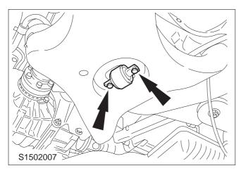
11. Detach the ABS sensor (one bolt).
